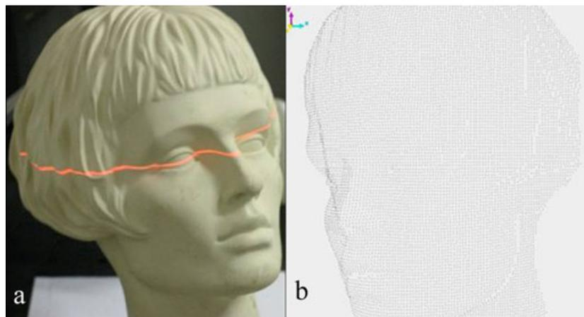
FIG. 1—The 3D optical digitizer measurement principle. (a) The deformation of the laser stripe induced by the object shape; (b) the whole point cloud of the inspected part.
