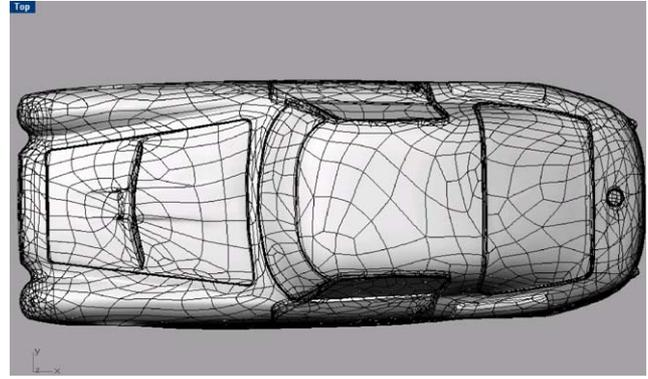
Fig. 7. Generation of the CAD models: patch layout.
