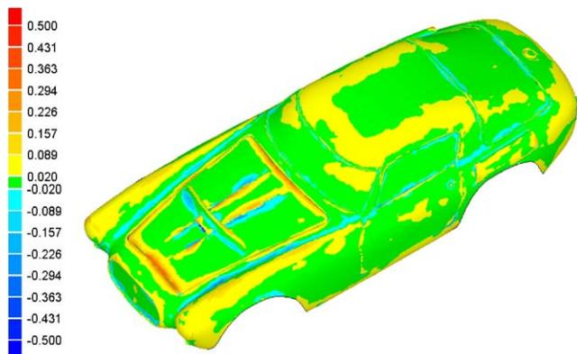
Fig. 8. Colour coded error map of the 8-control points model.
