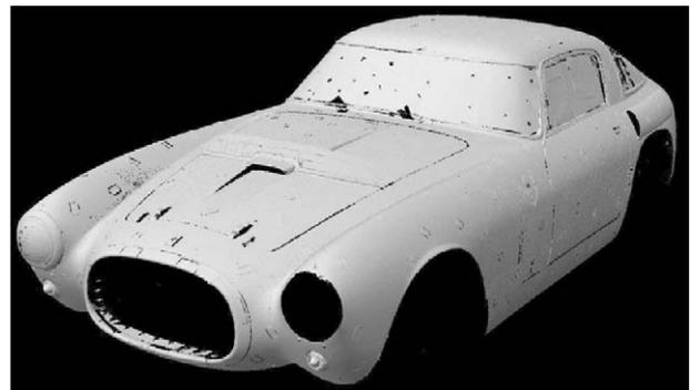
Fig. 5. Whole point cloud of the Ferrari 250MM.
