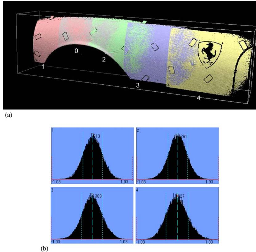
Fig. 4. Alignment of five adjacent point clouds: (a) visualisation of the aligned views; and (b) histograms of the error distributions.
