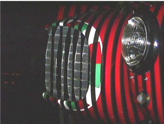
Fig. 3. Projection of one out of 11 patterns of the Grey Code-Phase Shift sequence on the car body.
