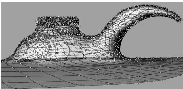
Fig. 9. CAD representation of the left-door handle.
