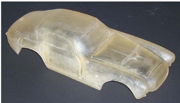
Fig. 10. 1:10 scaled replica of the Ferrari 250MM obtained from the 75 MB triangle mesh.
