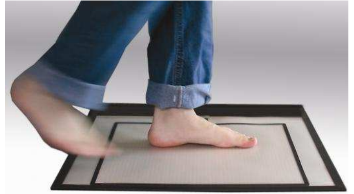
Fig. 2. The force platform used to measure the instantaneous position of the centre of pressure (COP)
